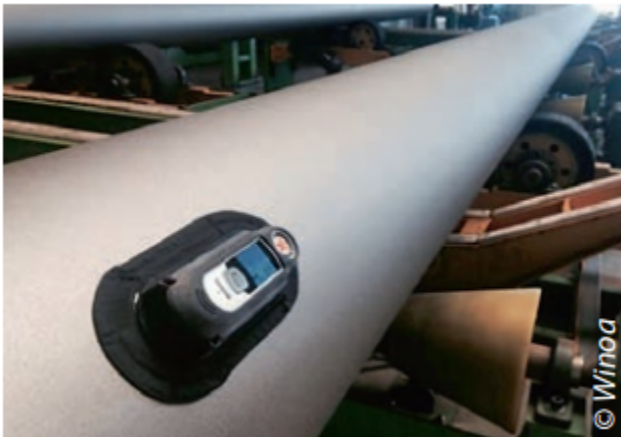
Practical use of the measurement device enables optimised blasting times by preventing the over - blasting
