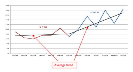
The conclusion is that desanding is at least the same as before with 10% less amps, so 10% less abrasive thrown. Comparative results obtained with WS390 & HPG8: Tons blasted with 1 ton of abrasive.
