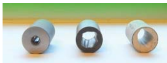
CERBIDE™ after 20 days Hardness: Rockwell A: 95.5 regular carbide after 3 days Hardness: Rockwell A: 92 alumina after 1 day Hardness: Rockwell A: 91
