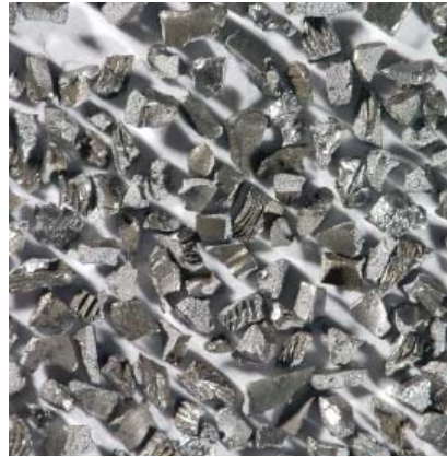
High-Chromium grit for specific blasting operations
