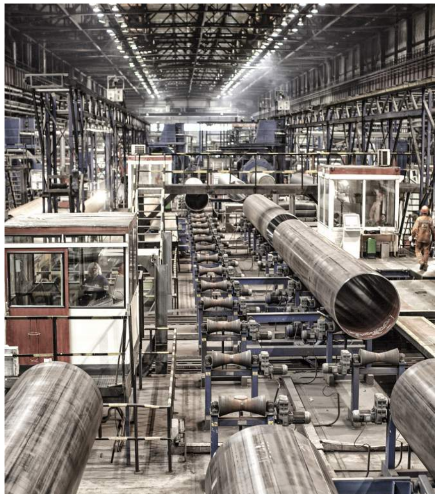
Large diameter steel pipes heading to the external blasting machine
