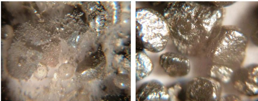
**Example of a non-efficient abrasive cleaning adjustment, resulting in a contaminated operating mix (left); a clean OM is shown, right.**
