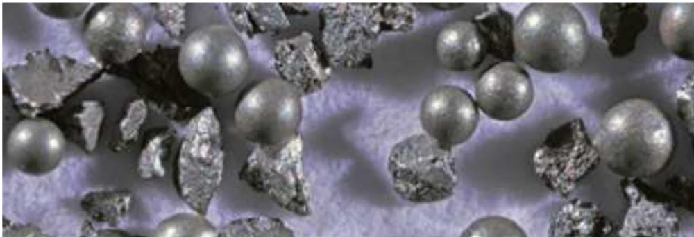
**Stainium is a high-performance steel abrasive for surface preparation.**
